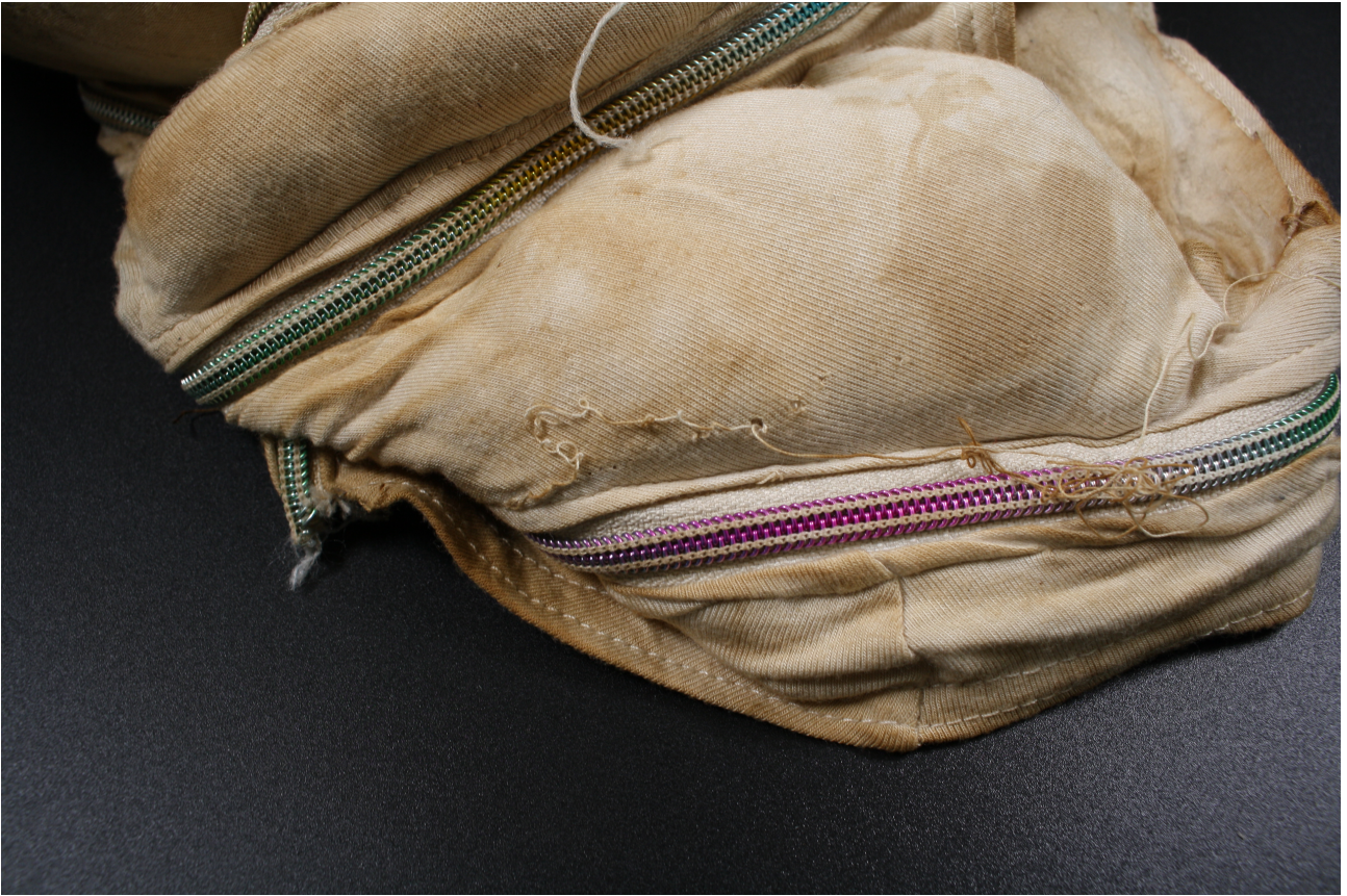
Figure 3 Details of loose threads
