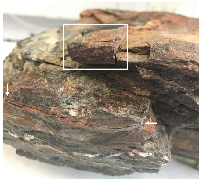
Fig.6 Long cracks (white arrows) and a loose piece (white rectangle).
