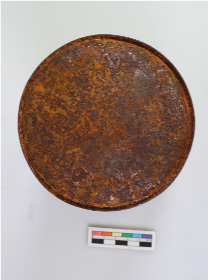
Figure 2. Top image of can. Shows the extent of the rust on the lid. The raised edge of the lid is visible, where the rust is mainly flaking from the surface.
